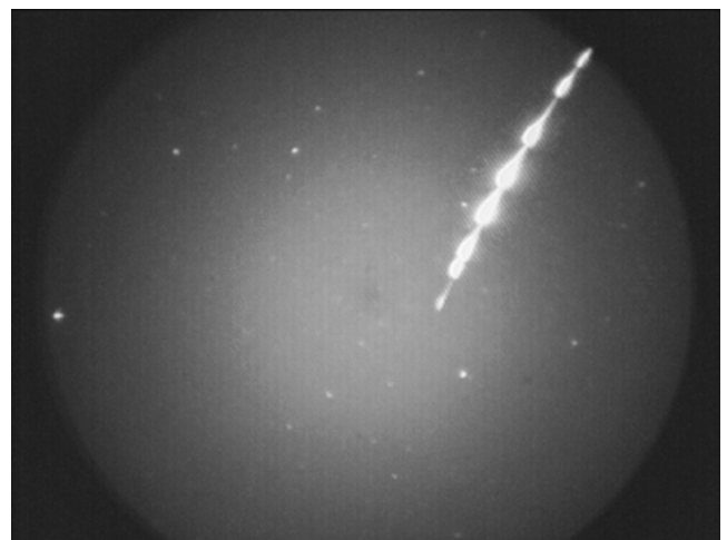
Figure 4 – Image taken with FIFIE from Utrecht, but equipped with a 200 mm, f/4 lens instead of the 50 mm lens. The brightest star left is \chi Draconis of magnitude +4, the weakest stars are of magnitude +8.
