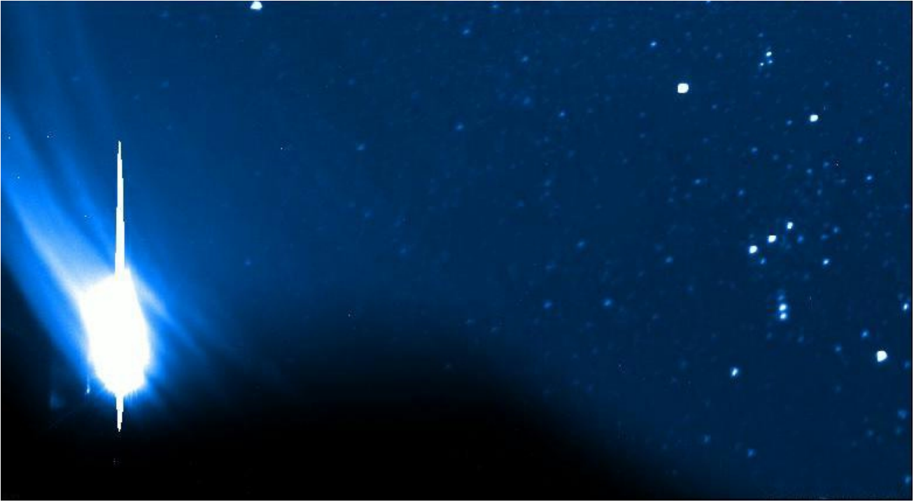
Figure 1 – A part of the CCD all-sky image of the 2003 January 27/28 fireball SPMN030101 registered from the El Arenosillo station in Huelva (INTA-LAEFF). It is important to note that the vertical brightest line is produced by CCD saturation and that the fireball trajectory deviates slightly from this.
